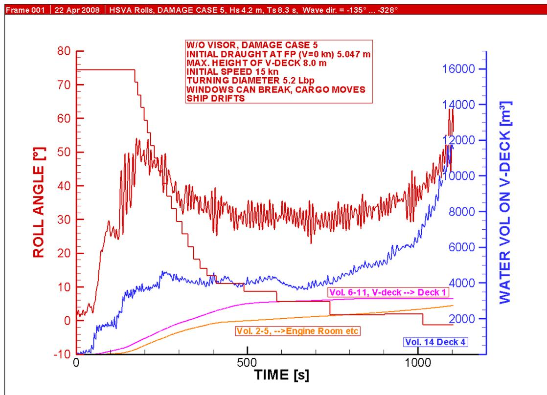
**Fig. 73** Time-history of roll used as a basis curve for the input in the evacuation simulations.
