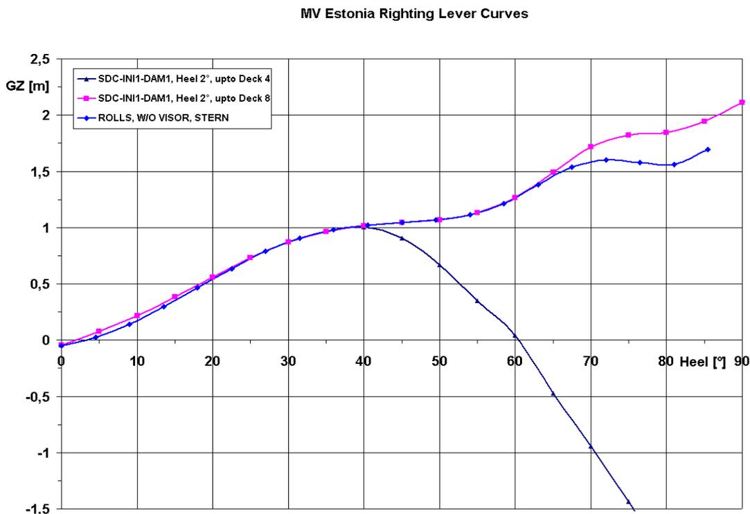
**Fig. A9** Righting lever curves for the *MV Estonia*
