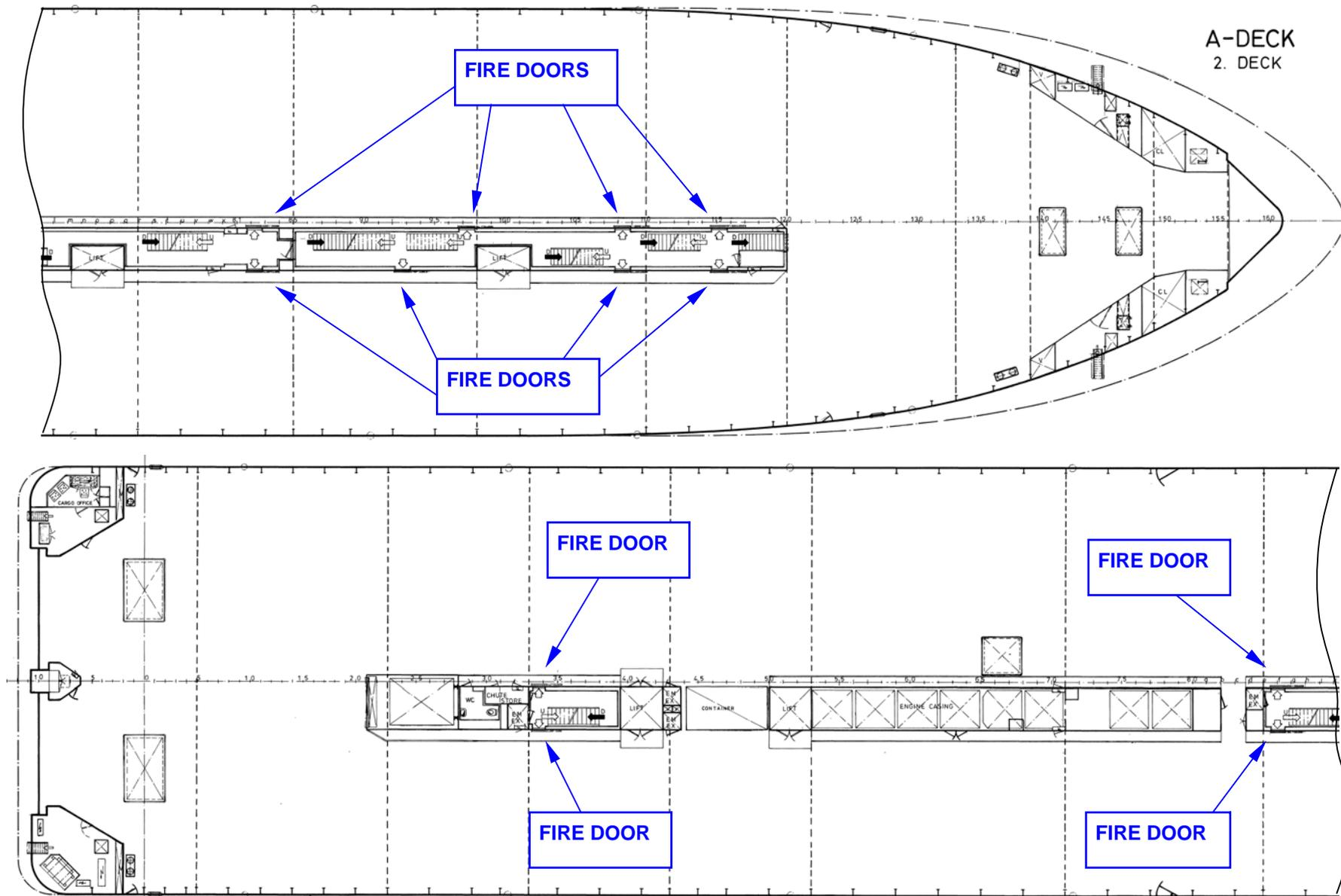
Fig. A13 Location of the fire doors in the center casing to the vehicle deck. Based on Jos. L. Meyer Drawing No: S590-02/3.
