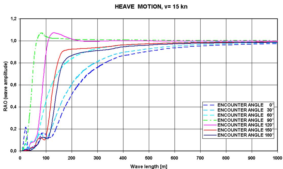
**Fig. A16** The Response Amplitude Operator for heave motion.
