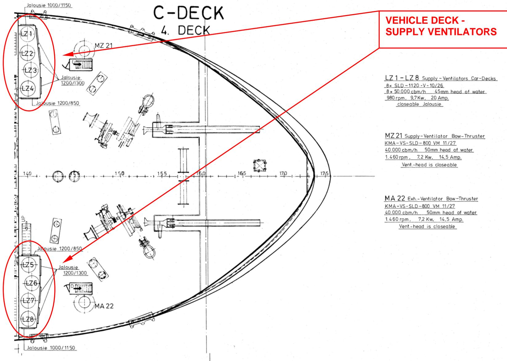
Fig. A11 Location of the supply ventilators to the vehicle deck. Based on Jos. L. Meyer Drawing No: S590-64/1.
