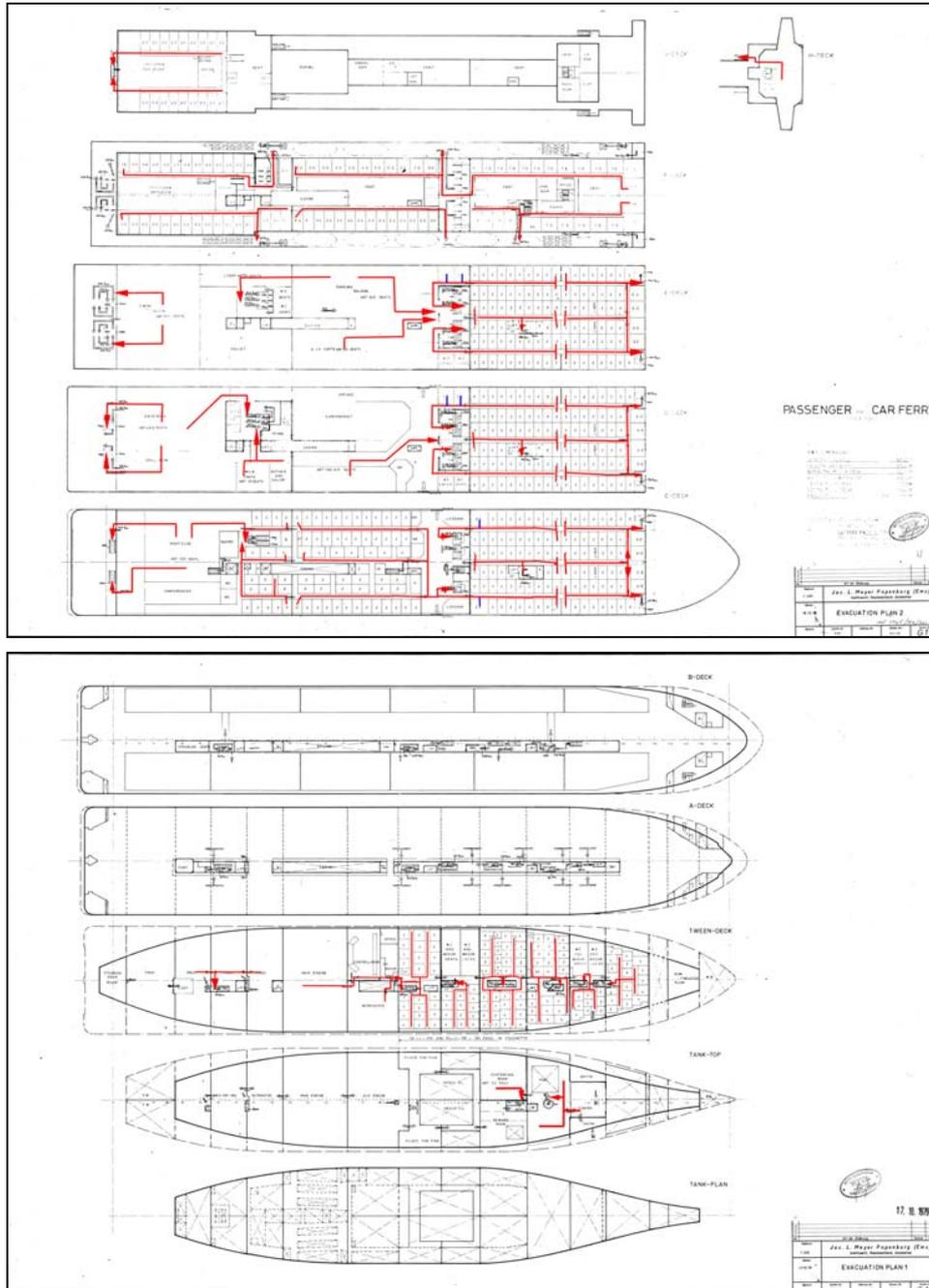
**Fig. 61** Egress routes for cases 1 and 2. The evacuation routes are indicated by red arrows. Few routes starting from crew cabins are blue, but merge in the corridor into the same red egress route.
