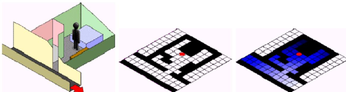
*A room and a small corridor as a simplified example. The geometry is transformed into cell informations. From the appointed exits, potentials spread according to free cells, following the given egress routes. The celltypes are used: walls, gradient of the blue color doors, stairs. marks the potential value.*
