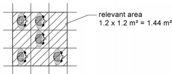
**Fig. 65** Example for the density calculation in a cellular grid.
