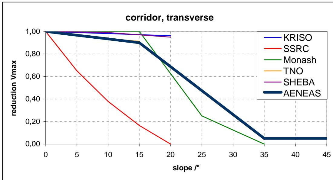
**Fig. 54** The speed reduction as a function of the transverse slope in a corridor. The model used in AENEAS is shown together with empirical data and the SSRC model (Valanto, 2006).
