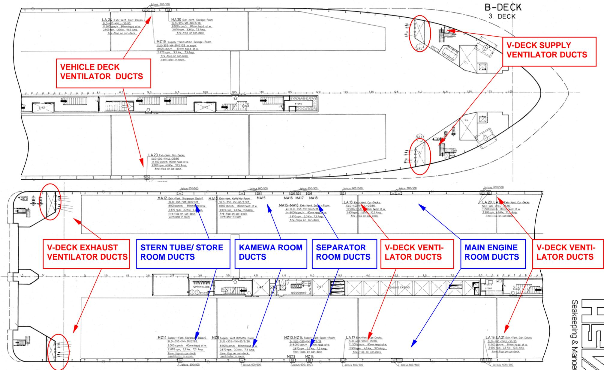
Fig. A10 Location of the ventilation ducts to the vehicle deck and to several spaces below the vehicle deck. Based on Jos. L. Meyer Drawing No: S590-64/1
