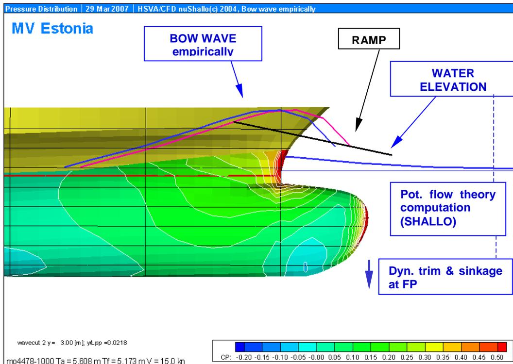
**Fig. A4** Water elevation at the bow.
