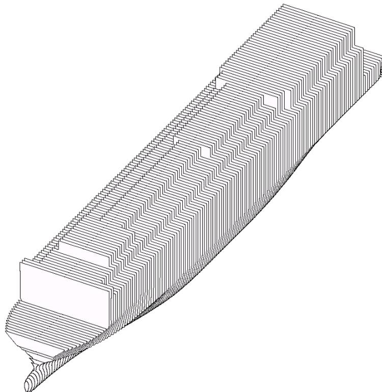
**Fig. A8** NAPA-Geometry of the *MV Estonia* without the visor used in computing the righting lever curves.
