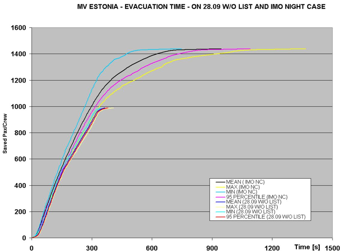
**Fig. 71** Comparison of the evacuation simulation of the standard IMO Night Case on *MV Estonia* and simulation of the real *MV Estonia* on 28.09.1994 without list. The IMO Night Case evacuation is symmetric to both sides of ship. In the real *MV Estonia* case the evacuation is asymmetric to the port side only.
