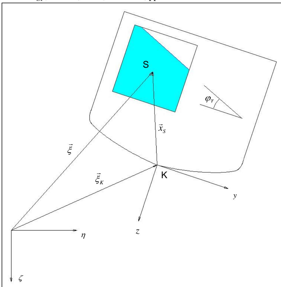
**Fig. A6** Definition sketch for a ship with a tank.
