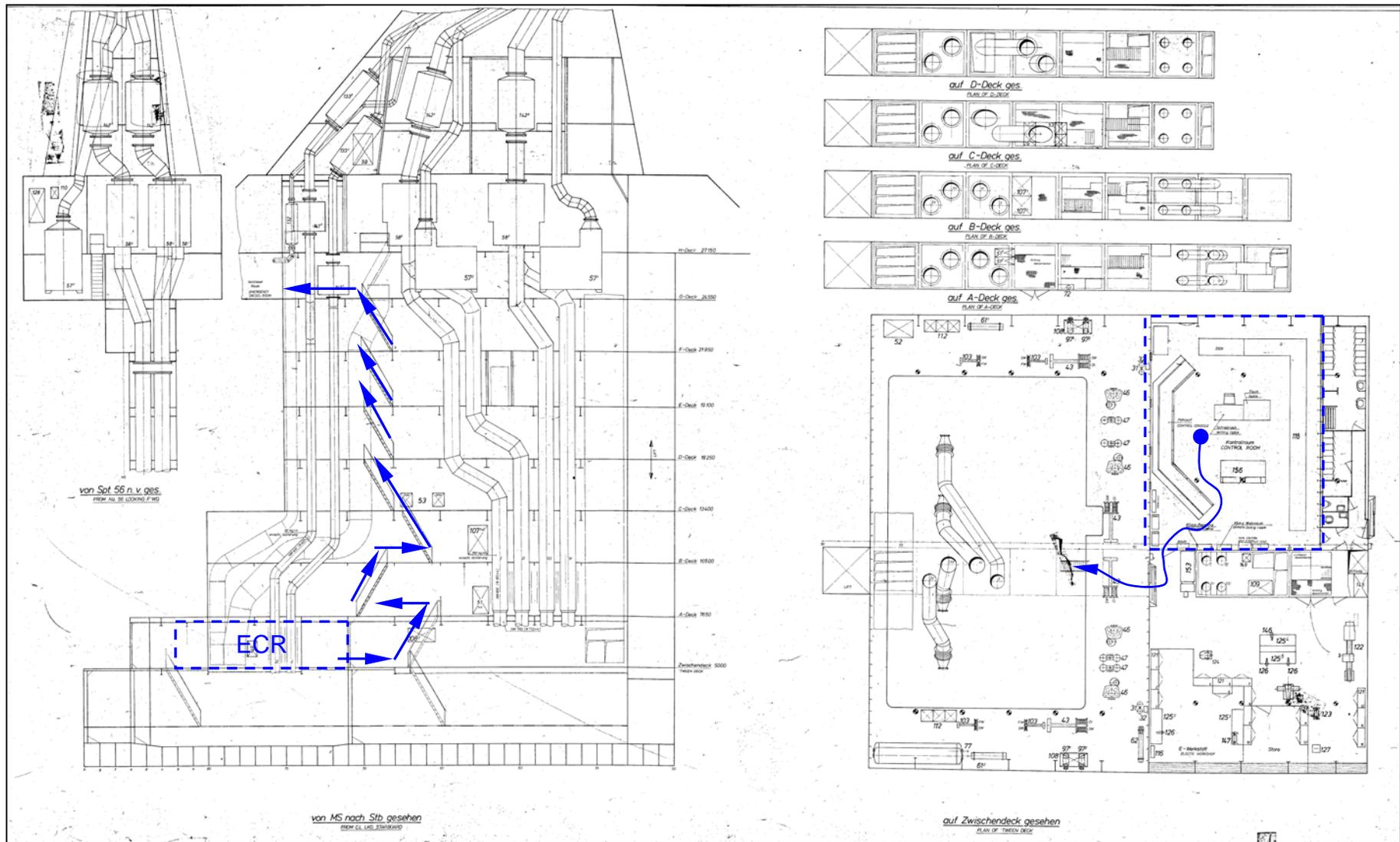
**Fig. 63** Extracts from the Jos. L. Meyer drawing No. MA500 showing also the egress route out of the ECR. The detail in the middle showing the exhaust pipes in the funnel is seen from the port side of the vessel looking to the starboard side.
