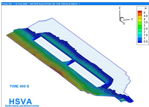
**Fig. 39b** Screenshots of the vehicle deck flooding according to the simulation with HSVA ROLLS at times 90, 120, 180, 240, 300, 360 and 400 s. The coloring expresses the water height on the deck perpendicular to the deck.
