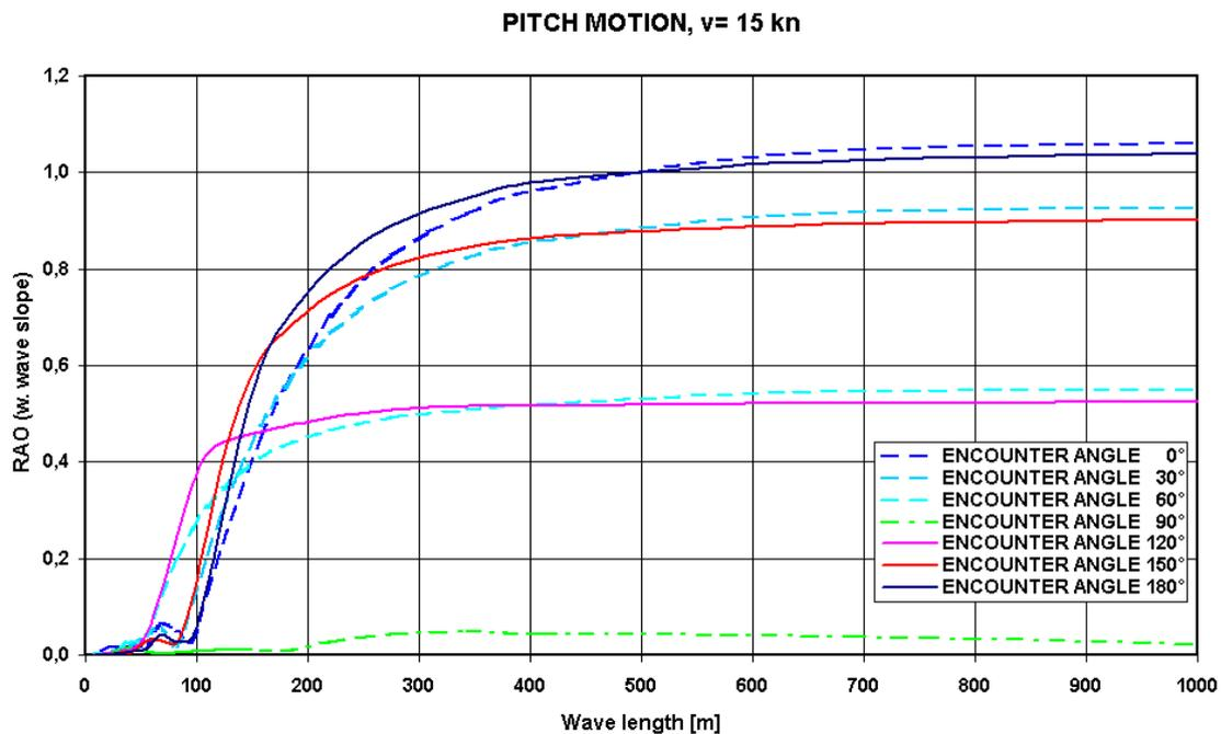
**Fig. A15** The Response Amplitude Operator for pitch motion.
