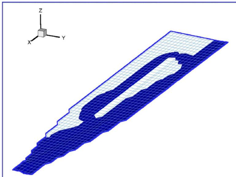
**Fig. A5** A momentary water elevation on the vehicle deck during the time integration of the numerical solution.
