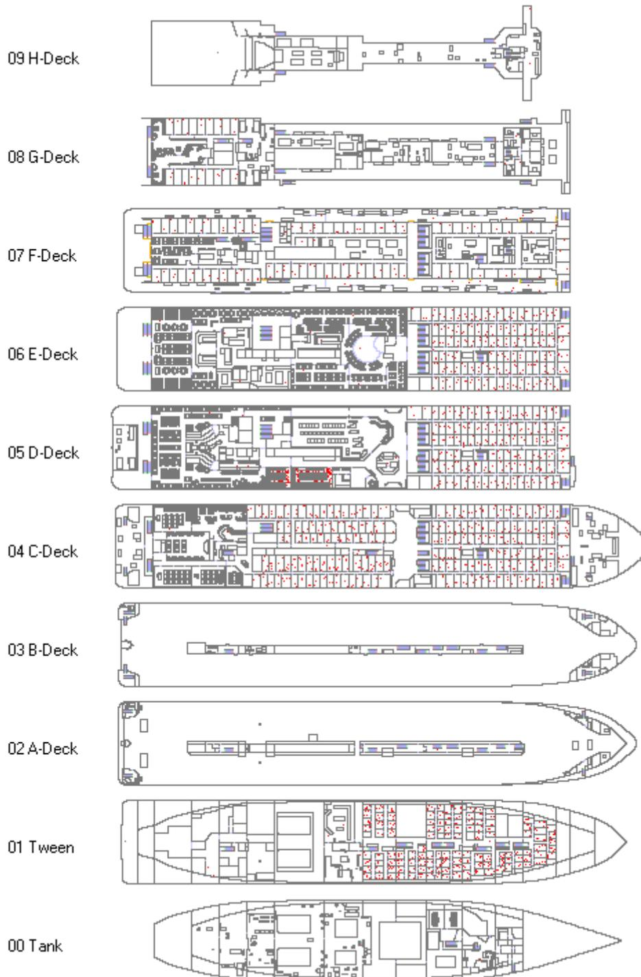
**Fig. 55** Cellular representation of the floor plan for scenario 1 (IMO Night Case). The red dots mark passengers.
