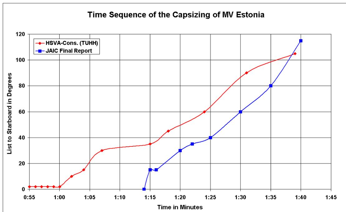
Fig. 67 Development of list to starboard during the *MV Estonia* accident.
