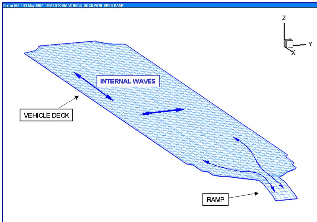
**Fig. A1** The numerical grid used to model the fluid motion on the vehicle deck and on the open ramp. Notice the center casing in the middle.
