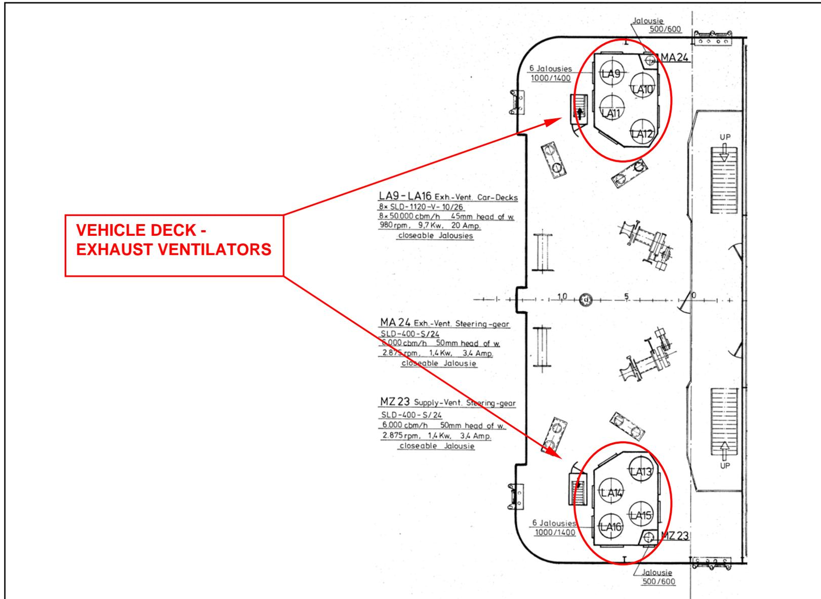
**Fig. A12** Location of the vehicle deck exhaust ventilators on the C-Deck. Based on Jos. L. Meyer Drawing No: S590-64/1.
